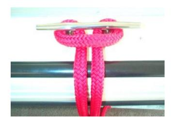
Attach your rope to your boat using the boat cleats as shown on the left. If you attach ropes to your rails you can assume there will be damage.
