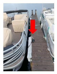
In the top left photo, note the placement of the cleat on the dock. This allows you to pull the boat back far enough to keep the front of the boat clear of the dock. You could also use the post at the end of the dock to pull the boat back using the loop in the right photo.
